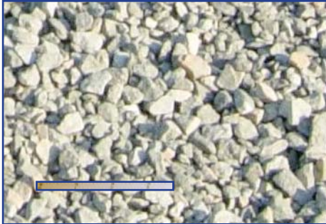
Figure 1: DOT-Certified 0.375-0.75-inch Miami Limestone aggregate from the Lake Belt (Source: LHC)
