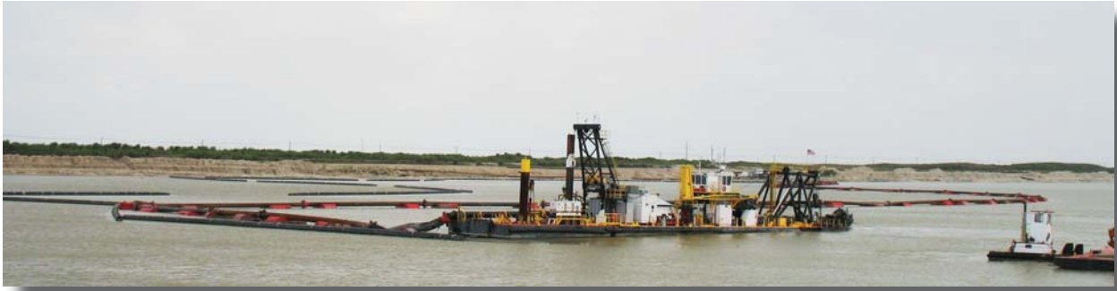
Figure 3: Floating sand dredge (Source: LHC)
