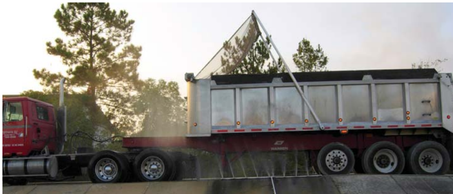
Figure 13: Tractor trailer combination dump truck in 3 axle configuration with a lightweight aluminum dump body (Source: LHC)
