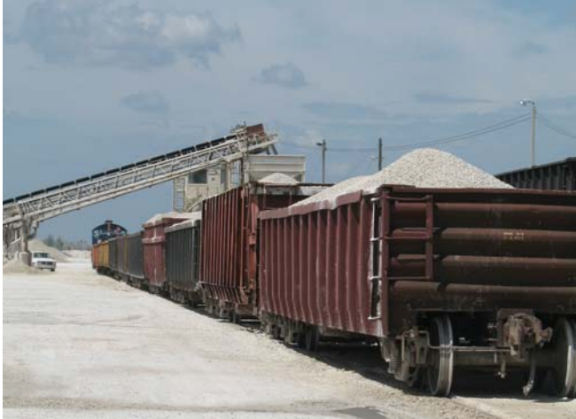
Figure 15: Hopper cars of 100-ton capacity being loaded at Rinker FEC Quarry (Source: LHC)
