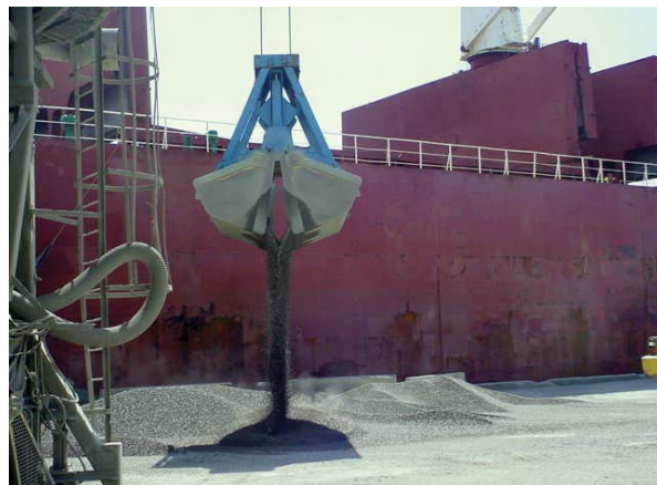
Figure 18: Unloading with shipboard equipment at Port Manatee (Source: Mark Gregory, FDOT)
