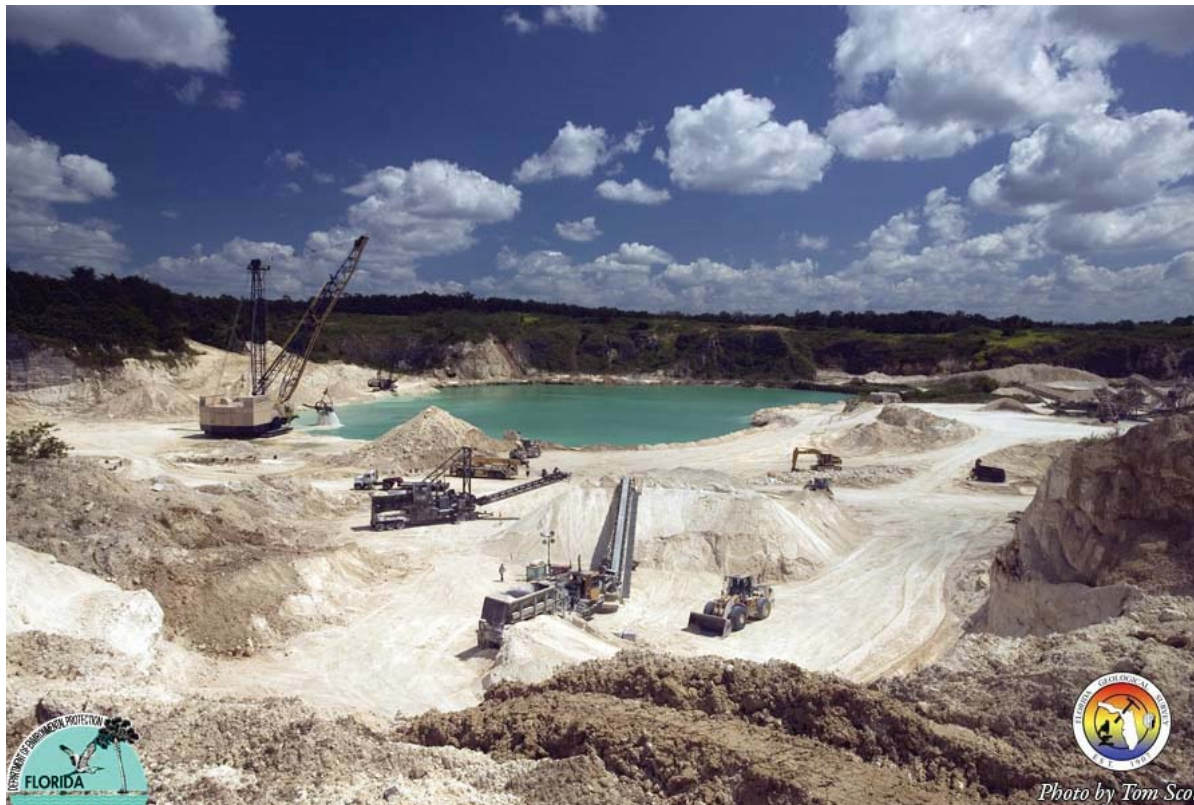
Figure 6: Small, “wet mining” operation where overburden and overlying limestone have been stripped to the top of the water table.
