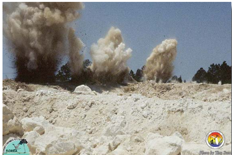
Figure 5: Breaking limestone by blasting (Source: FGS)
