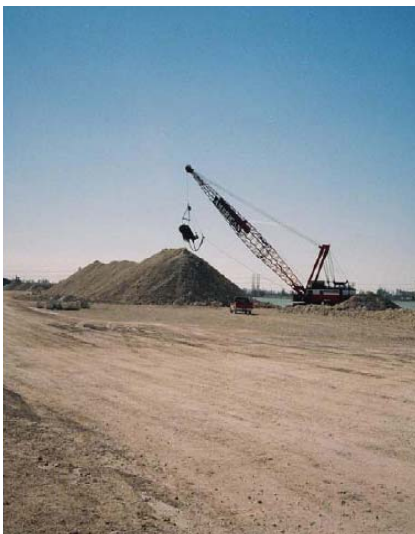
Figure 2: Dragline in operation in the Lake Belt (Source: LHC)
