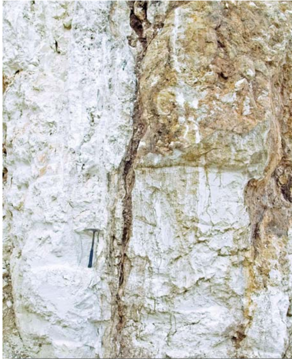
Figure 4: Fracture zones in the Ocala Limestone that have allowed chemical hardening of the formation
